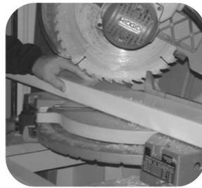
**Step 4:** If Z-Wedge is not required; subtract 1/8" per side (1/4" total) to allow space for the bracket base plates. Miter cut both the top and bottom rails, including aluminum reinforcement.
