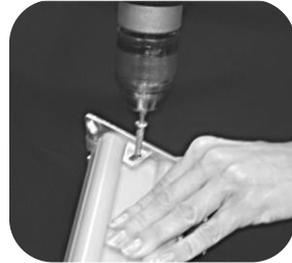
**Step 10:** After sliding bracket covers onto rail. Insert bracket plate into each end of top rail and secure plates to sides using (2) 1" stainless steel screws(provided). Pre-drill with 1/8" bit.
