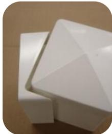
**22.5° Adaptor:** Used to attach VI Pro railing brackets at a 22.5° horizontal angle to Post. Deduct an additional 3/8" per side from rail in step 4.
