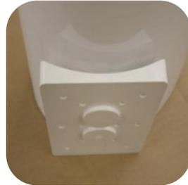
**8" Column Adaptor:** Used to attach Pro-Z railing bracket onto an 8" round column. Deduct an additional 1/4" per side from rail in step 1.
