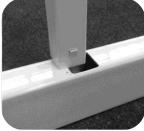
Step 6: Option 1. Routed Foot Block. Cut 6" square foot spindle down to 1-5/8" longer than desired undercut. Not required on kits less than 48" long. Newer kits will not have hole pre-routed. Cut a 1-1/2"x1-1/2" hole in center of underside of bottom rail. Note: Rails longer than 8' in length require 2 foot blocks.
