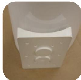
**8" Column Adaptor:** Used to attach Pro-Z railing bracket onto an 8" round column. Deduct an additional 1/4" per side from rail in step 4.
